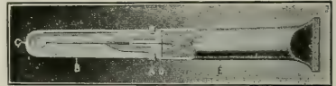
Fig. 1. The Greeley unit. Twist off the cap B, withdraw the stylet C, and the unit is ready for use.
